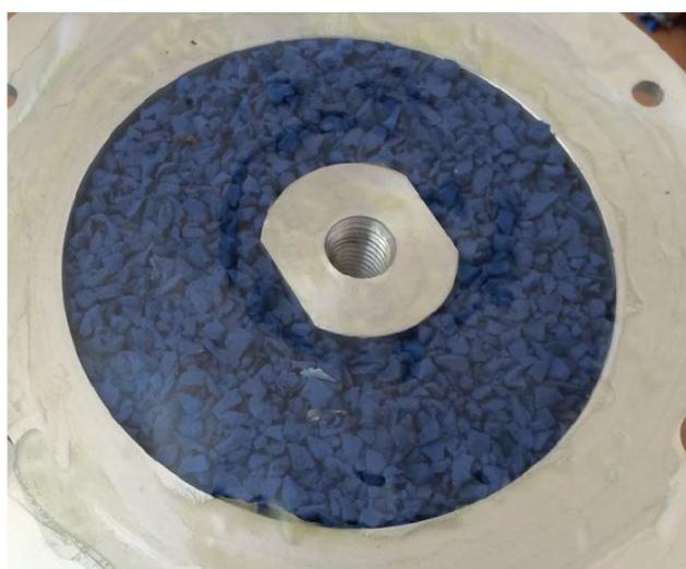
**Figure 7.** SVPP damper with EPDM grains.
