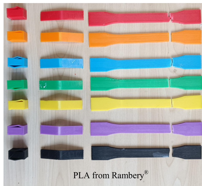
Figure 10. Broken PLA specimens from Rambery® after confirmation test.
