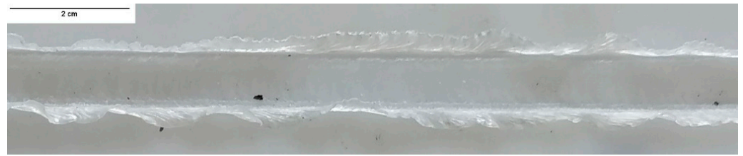
Figure 3. Flash defect on the surface of the weld PE_1140_60.
