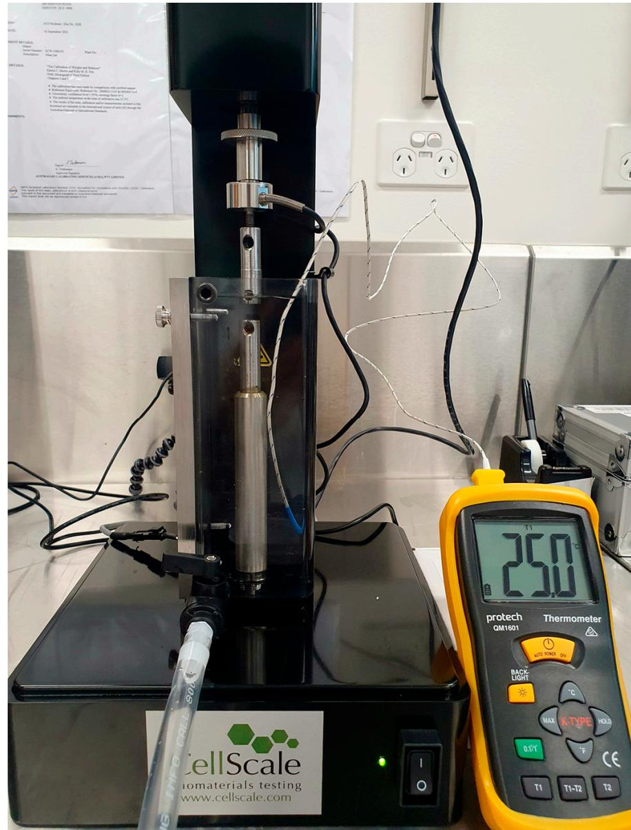
**Figure 5.** Photograph of UniVert microtensile test setup used.
