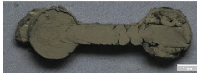
Figure 6. Jetting problem during the injection molding step. Reproduced with permission from reference [33], copyright © 2014 Elsevier B.V.
