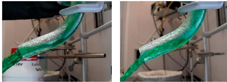
**Figure 10.** Water (left) and SCN (right) in SLA printed channel.
