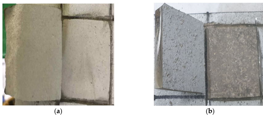
Figure 8. Interfacial failure mode according to surface treatment conditions. (a) Control; (b) SH.
