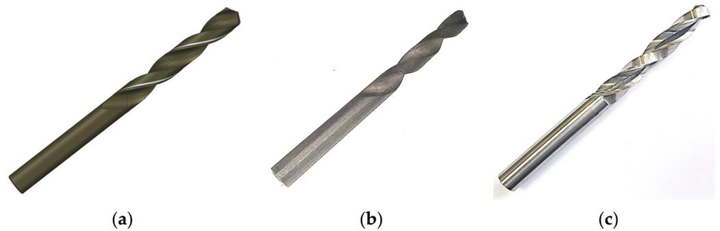
**Figure 2.** Stages of the 3D printing of the twist drill bit: (a) 3D model, (b) drill bit before grinding, (c) drill bit after grinding.
