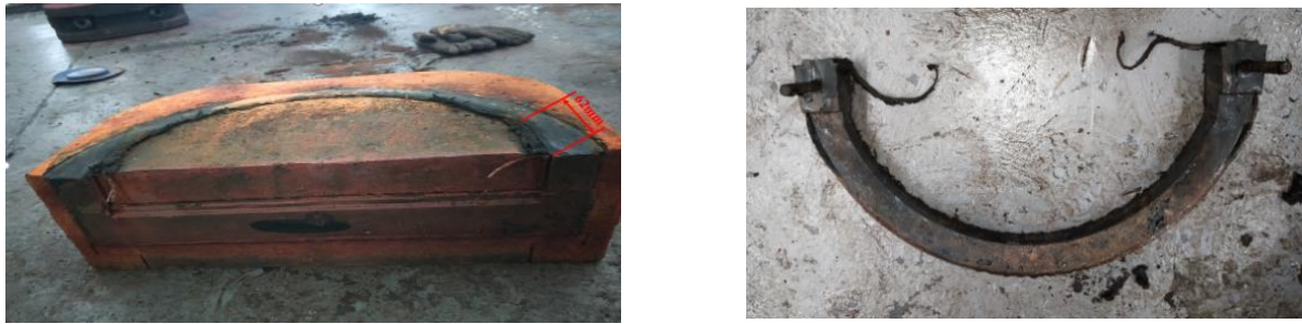
Figure 4. Rubber core failure.
