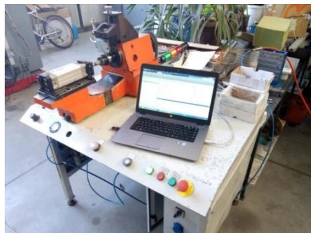
**Figure 2.** Experimental device for measuring ball bearing vibrations.
