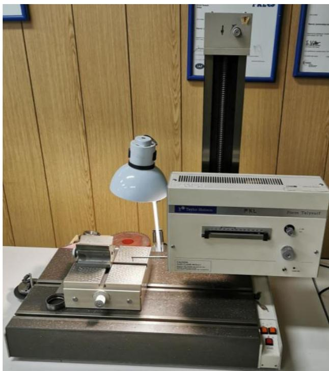
Figure 1. Taylor–Hobson Form Talysurf 112/1849 Device.
