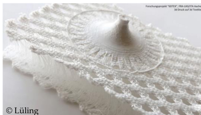
Figure 17. Warp knitted spacer fabric combined with a 3D-printed object for lightweight building components [81].
