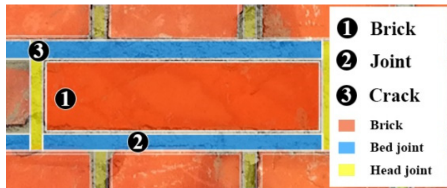
Figure 9. Partition of the masonry into elements ready for modeling.
