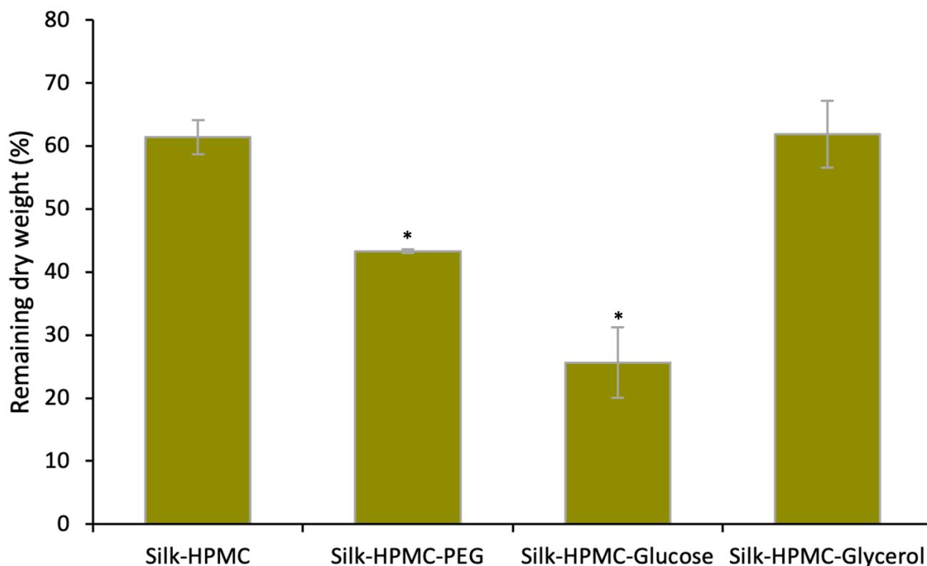
**Figure 1.** The remaining dry weight (%) from a degradation experiment of silk-based discs. Discs were immersed in PBS pH 7.4 for 7 days at 37 °C. Silk-HPMC-Glycerol showed the combined properties of lower degradation and a better ability to hold its shape. Two-way ANOVA showed significant differences among the groups. The Student's *t*-test was applied to evaluate the extent of differences between Silk-HPMC and other discs. \* indicates  $p < 0.05$ .
