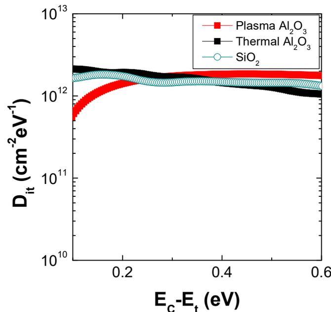
**Figure 3.**  $D_{it}$  distribution of T- $\text{Al}_2\text{O}_3/\text{SiO}_2(\text{IL})/3\text{C-SiC}$  and PE- $\text{Al}_2\text{O}_3/\text{SiO}_2(\text{IL})/3\text{C-SiC}$  MOS capacitors in comparison with the analogous  $\text{SiO}_2/3\text{C-SiC}$ .
