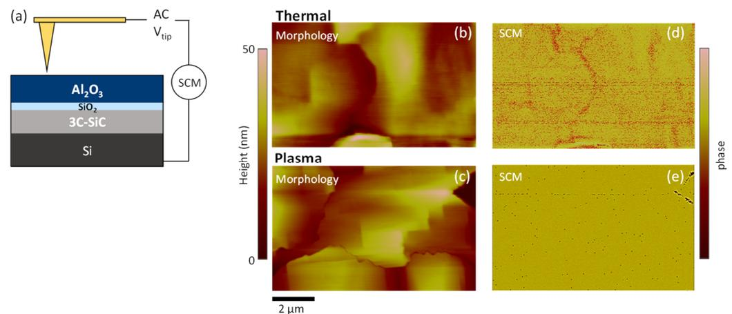
**Figure 5.** Schematic of the SCM experimental setup (a). AFM morphology of T- $\text{Al}_2\text{O}_3/\text{SiO}_2/3\text{C-SiC}$  (b) and PE- $\text{Al}_2\text{O}_3/\text{SiO}_2/3\text{C-SiC}$  (c). SCM maps of T- $\text{Al}_2\text{O}_3/\text{SiO}_2/3\text{C-SiC}$  (d) and PE- $\text{Al}_2\text{O}_3/\text{SiO}_2/3\text{C-SiC}$  (e).
