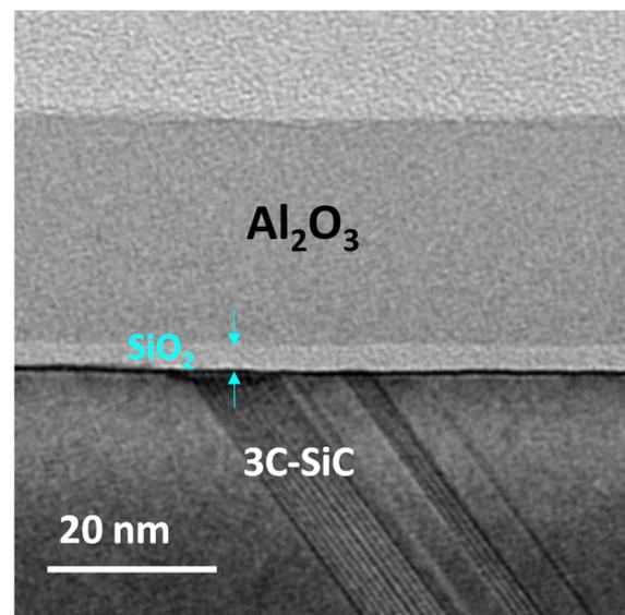
**Figure 1.** Cross-section TEM image relative to T- $\text{Al}_2\text{O}_3/\text{SiO}_2/3\text{C-SiC}$ .
