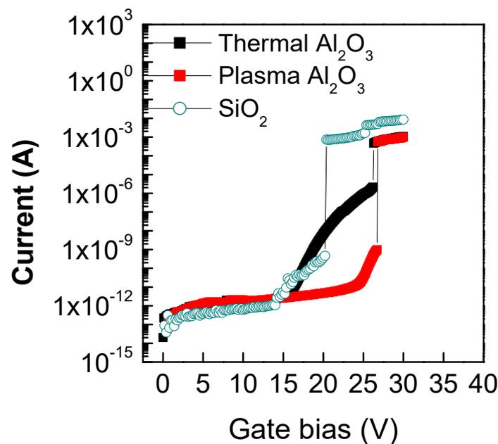
**Figure 4.** I-V measurements of T- $\text{Al}_2\text{O}_3/\text{SiO}_2/3\text{C-SiC}$  and PE- $\text{Al}_2\text{O}_3/\text{SiO}_2/3\text{C-SiC}$  MOS capacitors in comparison with the analogous  $\text{SiO}_2/3\text{C-SiC}$ .
