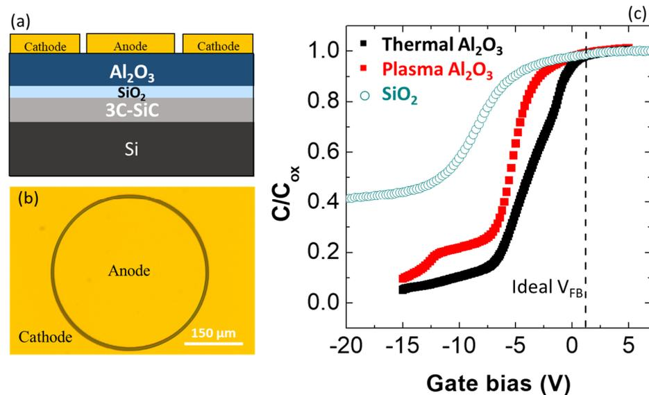
**Figure 2.** Schematic cross-section of the  $\text{Al}_2\text{O}_3/\text{SiO}_2/3\text{C-SiC}$  MOS capacitor (a) and top-view microscopy image of a MOS capacitor (b). C-V curves of T- $\text{Al}_2\text{O}_3/\text{SiO}_2(\text{IL})/3\text{C-SiC}$  and PE- $\text{Al}_2\text{O}_3/\text{SiO}_2(\text{IL})/3\text{C-SiC}$  MOS capacitors in comparison with the analogous  $\text{SiO}_2/3\text{C-SiC}$  (c).
