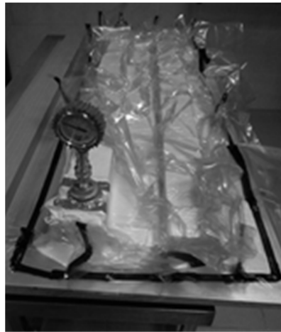
Figure 1. Process of manufacturing composite samples—vacuum package.
