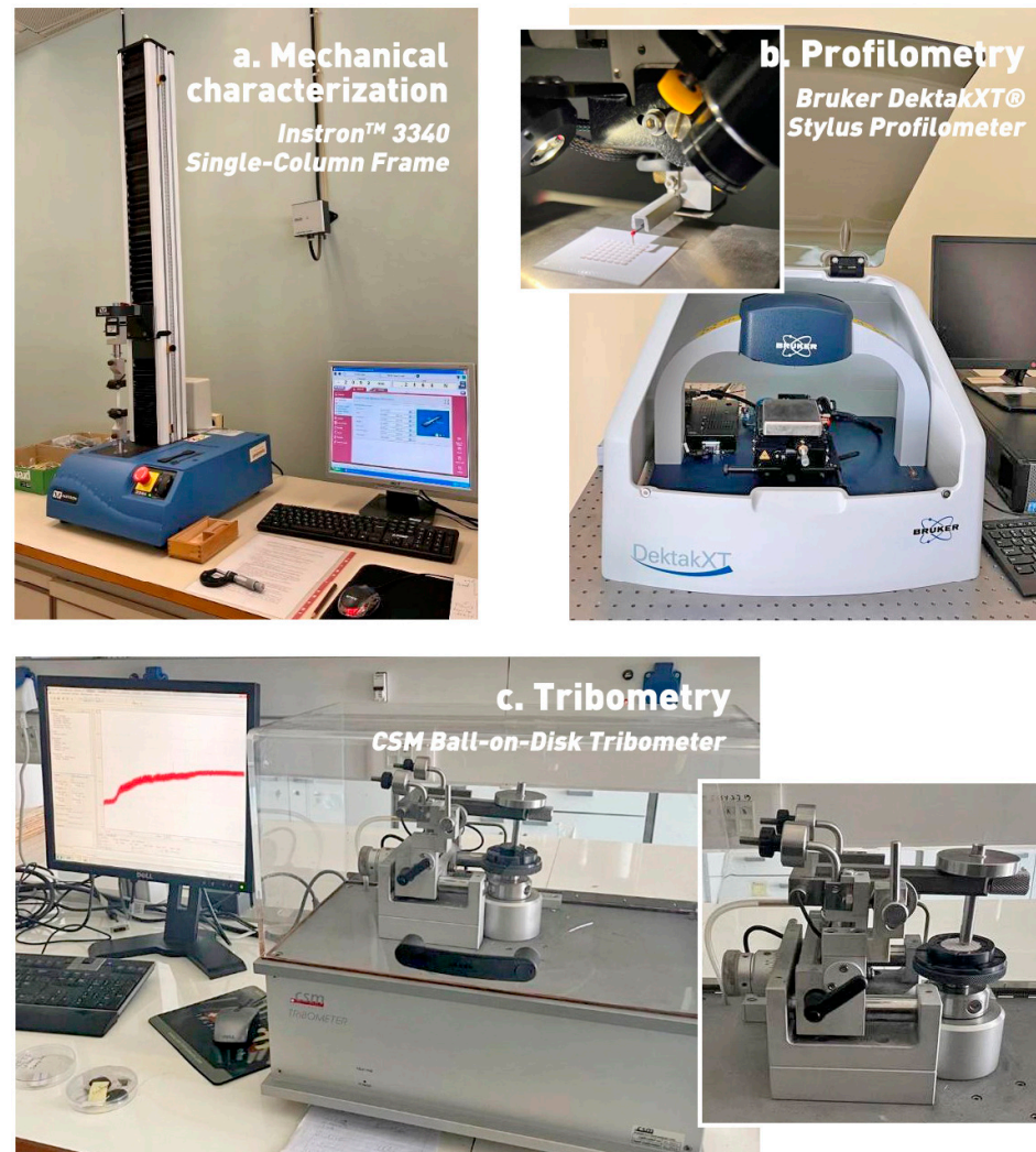
Figure 2. Main instrumentation used for (a) mechanical testing, (b) surface topography and roughness and (c) tribometry.
