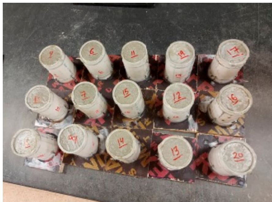
Figure 8. UCS shotcrete specimens prepared on 100 mm height and 50 mm diameter molds.
