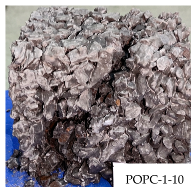
Figure 13. Failure mode of FOPC.
