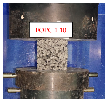
Figure 7. Test of the compressive strength of FOPC.
