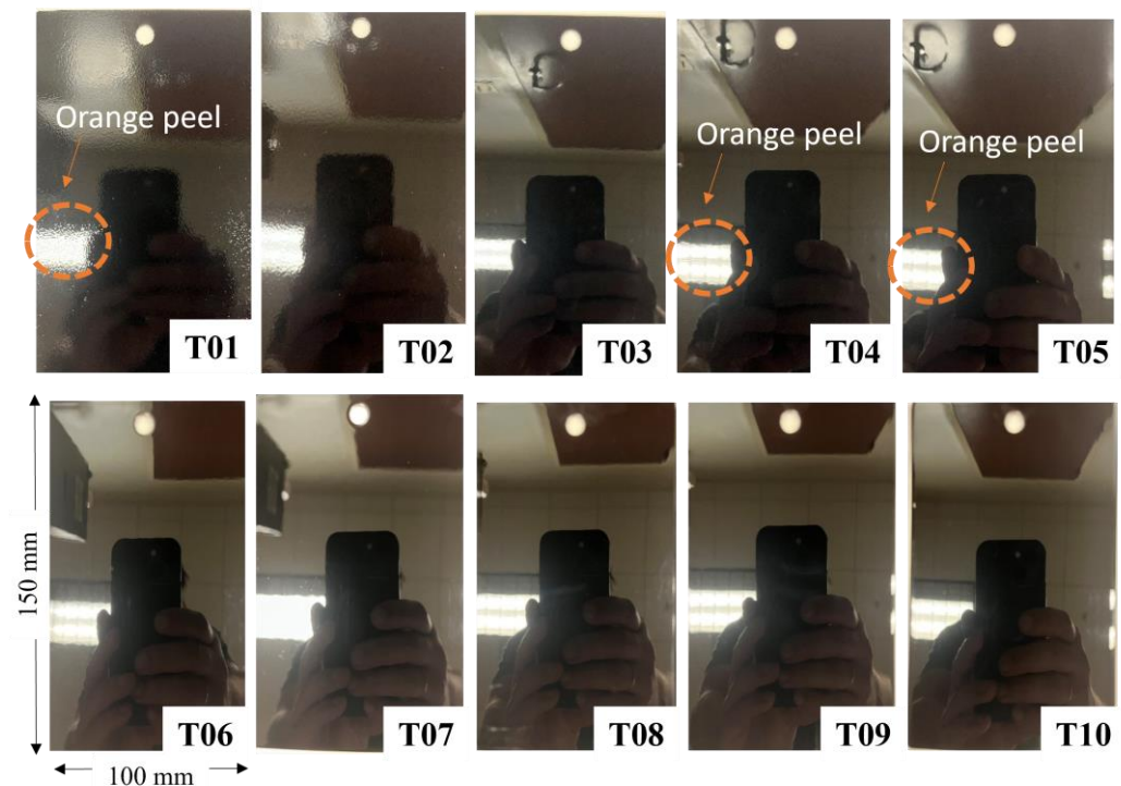
Figure 1. Images of PCI visual smoothness standards captured by an iPhone under non-ideal lighting conditions. Circular regions shown in T01, T04, and T05 illustrate the reflected image distortion caused by the severity of the orange peel.
