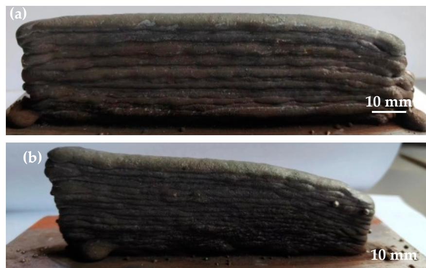
Figure 15. Macroscopic morphology of the as-deposited wall: (a) CMT, (b) CMT+P.
