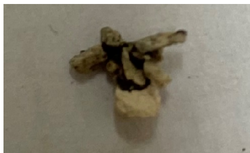
Figure 9. Example of sinter produced in the reactor, experiment 11 (diameter approximately 6 mm), which caused defluidization of the bed and problems with the feeder operation.
