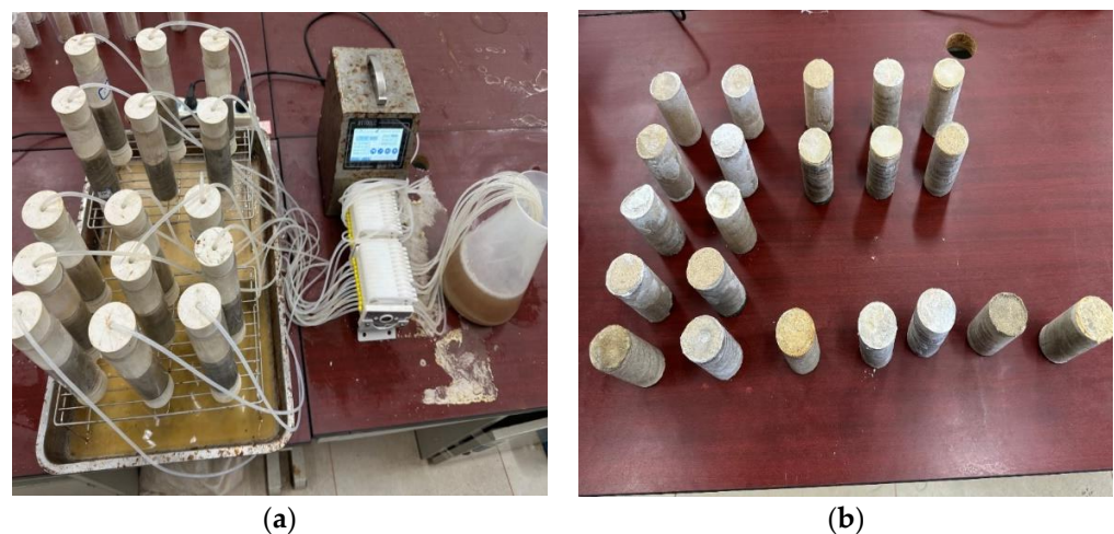
Figure 4. Grouting sampling process: (a) peristaltic pump grouting; (b) specimen after drying.
