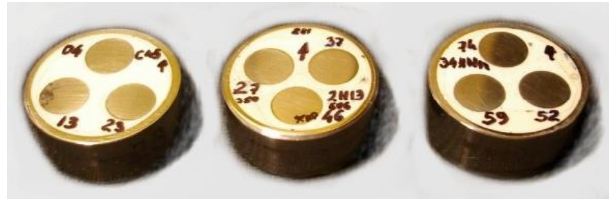
Figure 8. Specimens prepared for deriving characteristic values of forces P^* by means of indentation using Vickers probe.
