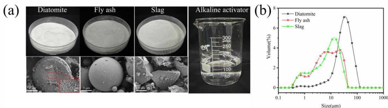
Figure 1. (a) Morphology of the raw materials and (b) particle size distributions of the precursor and diatomite.
