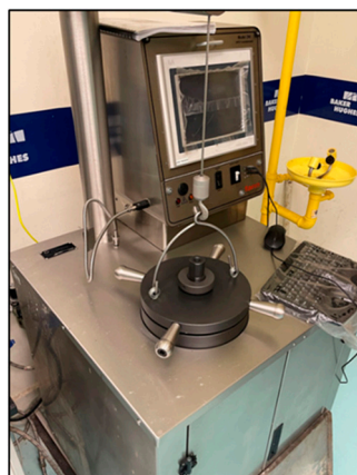
Figure 3. Consistometer For Thickening Time Test.
