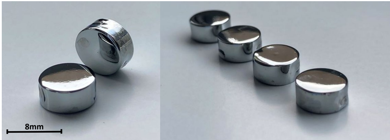
Figure 6. Macro-image of the titanium samples after EP.
