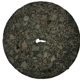
Figure 12. Pre-cracked asphalt mixture specimen with multi-grain aggregate ( D = 2.36 mm and 4.75 mm).
