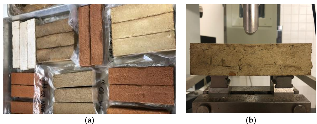
Figure 5. Standard prismatic specimens of the three earthen plasters (a); specimen being tested for flexural strength (b).
