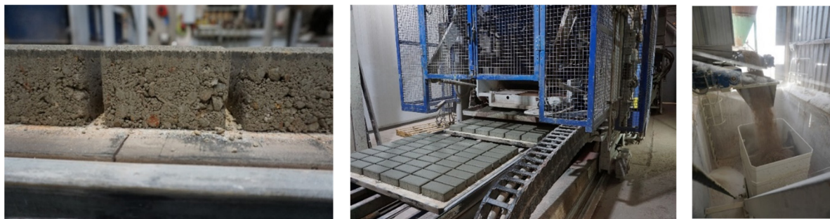
Figure 3. Manufacture of paving blocks, under industrial conditions.
