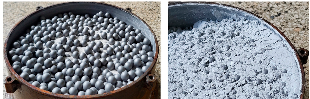
Figure 9. View of the chamber with 17.5 mm grinding media and material before grinding (on the left) and after 40 min of grinding (on the right).
