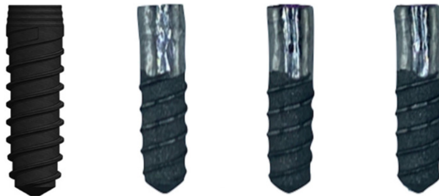
Figure 3. As-received dental implant and three examples of the implant treated by implantoplasty.
