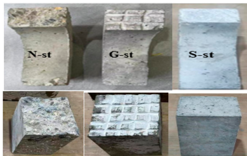
Figure 2. Surface treatment techniques adopted in this study.
