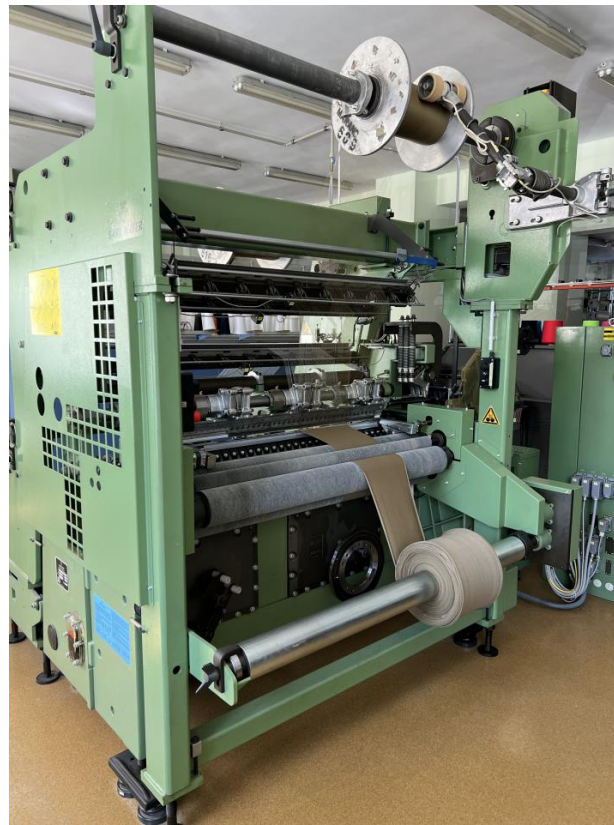
Figure 4. The HKS 3 warp-knitting machine from Karl Mayer, with needle number NE = 28 .
