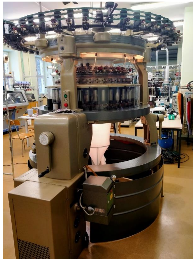
Figure 3. Cylindrical double-bearing crochet machine from Mayer & Cie (cylinder diameter = 30''; gauge pitch = 1.27 mm; needle number, NE = 20 ; number of needles, L = 2 \times 1872 ).
