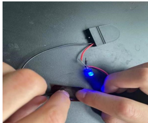
Figure 12. Illustration of polyimide film coated with conductive ink sintered at 300 °C.
