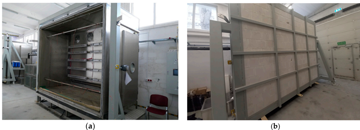
Figure 5. Artificial weathering chamber, view: (a) before assembling the test model (exposed heat radiators and spray nozzles), (b) after installing the test model exposed (aerated concrete wall as a substrate).
