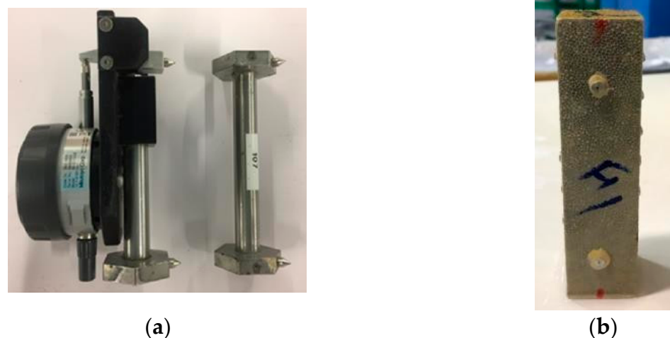
Figure 2. The extensometer and calibration section used to measure the variation in length (a); the mortar prism with a pair of pins fixed on one of the sides (b).
