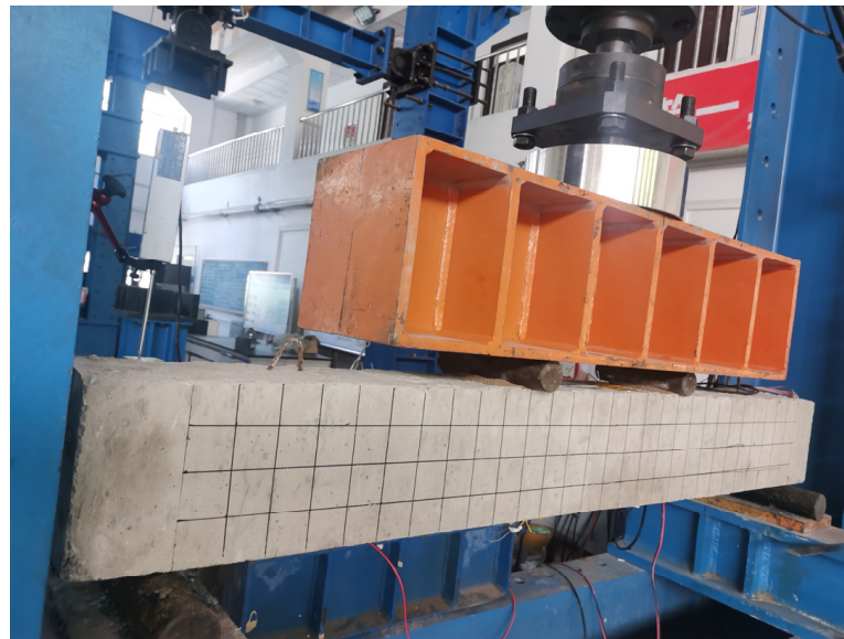
Figure 6. Four-point bending test setup.
