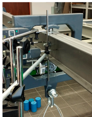
Figure 4. (a) Test bench diagram: 1—test model 2C, 2—support bearing, 3—support structure, 4—steel ball, 5—sling frame, 6—load platform, 7—weights; (b) Photograph of the sling frame; (c) Photograph of the support bearing.
