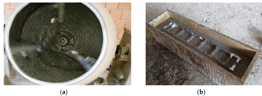
Figure 10. The cast of HPC: (a) pan mixer; (b) casting concrete in mold.
