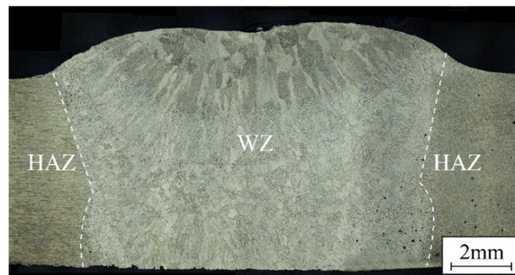
Figure 5. Macrostructure of single TIG-repaired joint.
