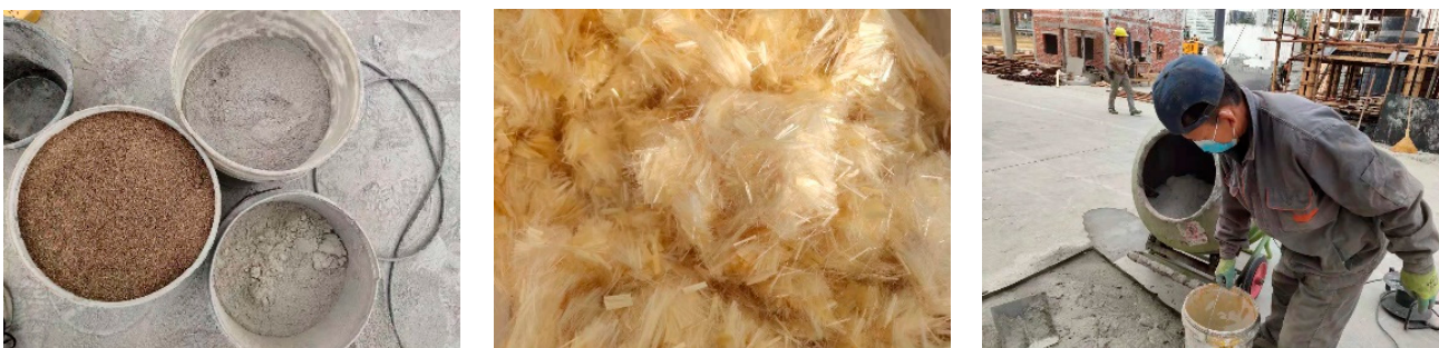
Figure 6. FRCM materials and mixing process.
