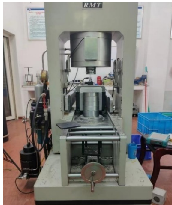
Figure 2. RMT-150 rock mechanics test pressure testing machine.
