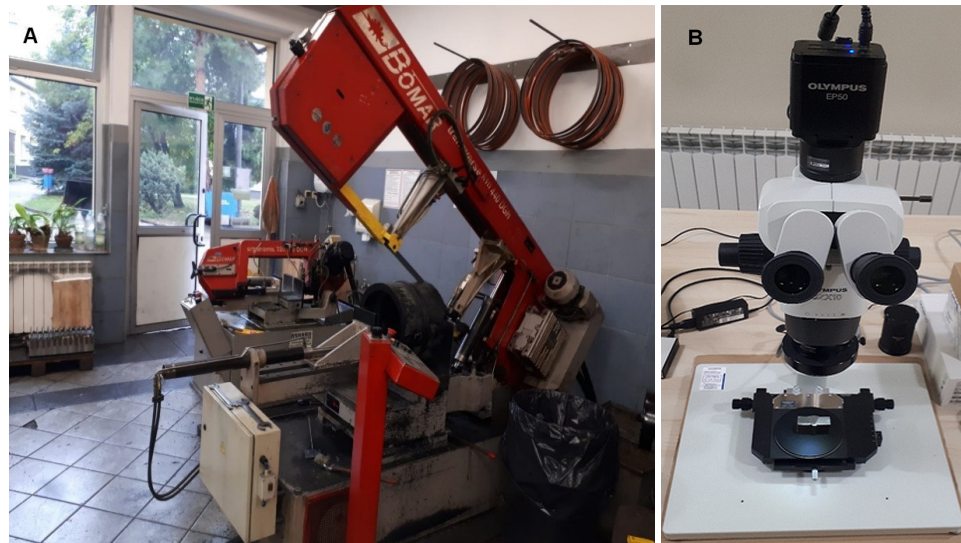
Figure 6. Instruments used to prepare samples and perform metallographic tests: (A) a Bomar saw model transverse 610.440 DGH used to cut the plates and (B) a station for taking photographic images of the scraps taken (Olympus SZX 10 stereoscopic microscope with EP50 camera).
