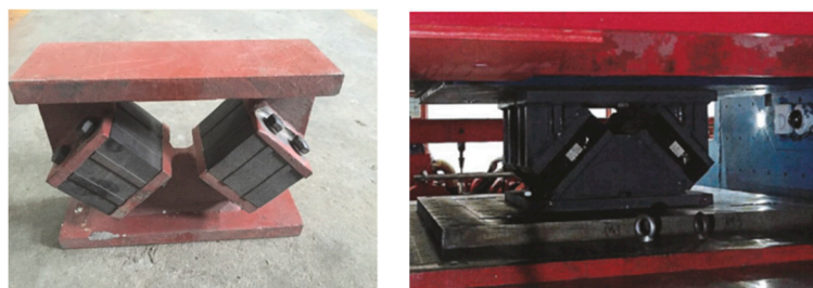
Figure 1. Test specimen of low-stiffness and high-damping rubber bearing.
