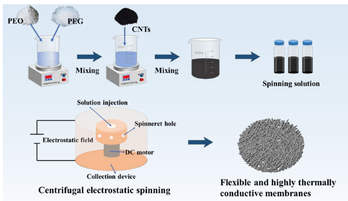
Figure 1. Centrifugal electrostatic spinning for the preparation of flexible and highly thermally conductive phase-change thermal storage membranes.
