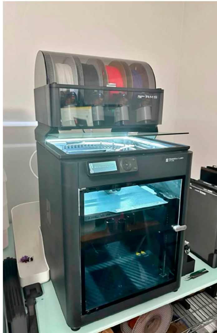
Figure 4. FDM 3D printer with enclosed chamber.
