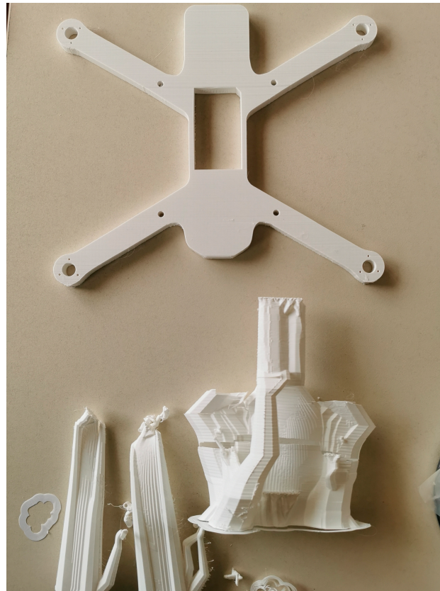
Figure 2. Drone frame upon the support structures' removal process completion.
