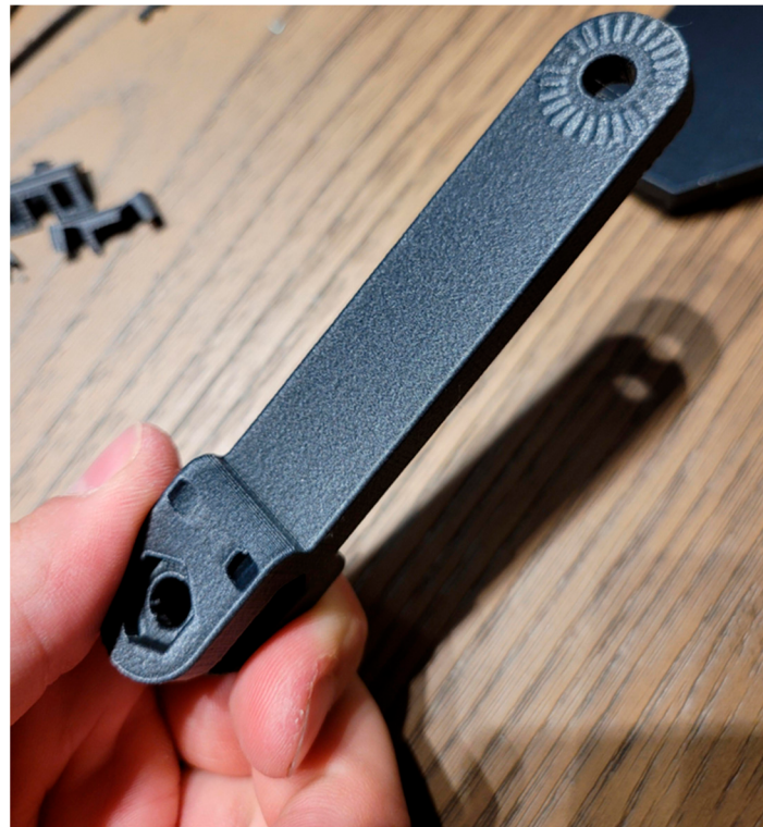
Figure 3. Three-dimensional printed part made out of carbon-fiber-reinforced PLA material.
