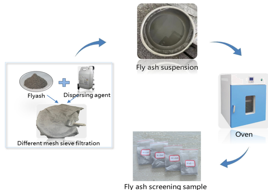
Figure 2. Preparation process of fly ash with different particle size.
