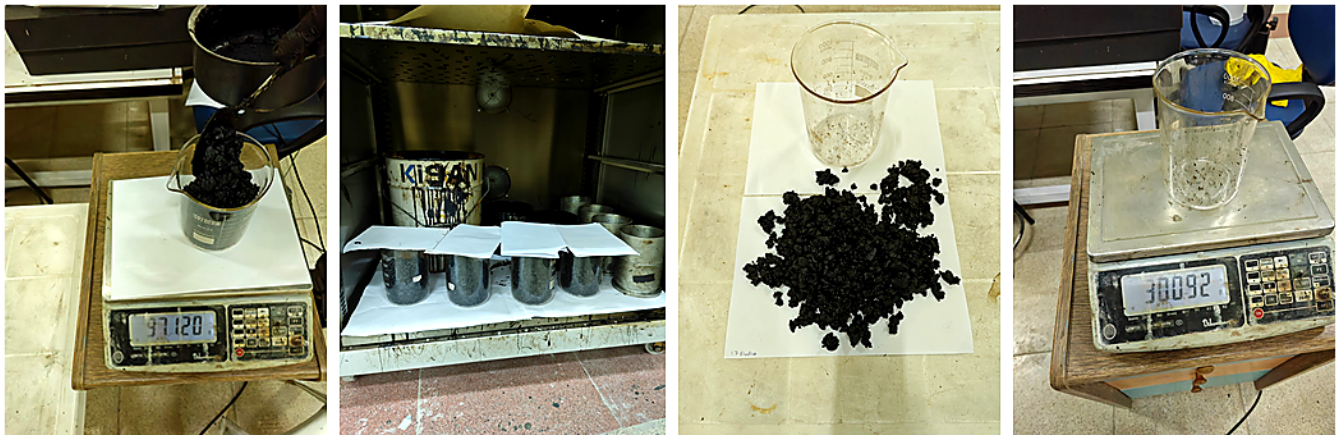
Figure 7. Stages of the bitumen drain-down test.
