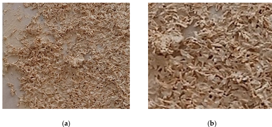
Figure 3. The appearance of a PRH-BG applied on a concrete surface. (a) Overview of the PRH-BG; (b) detail of the PRH-BG (2 \times ).
