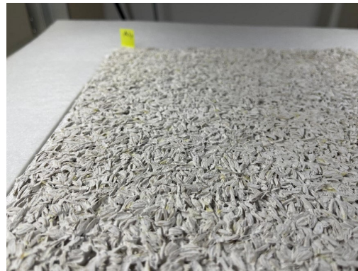
Figure 5. The sample with the tested PRH, placed in the thermal conductivity determination equipment with a perimeter, thermally insulating frame made of recycled PE non-woven material, in order to reduce thermal bridges.
