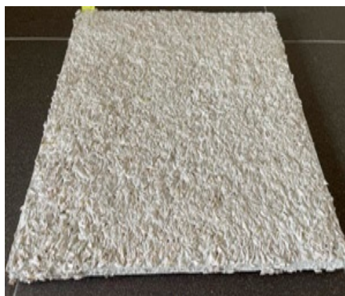
Figure 4. The appearance of a PRH applied on a plasterboard.
