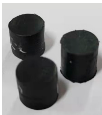
Figure 1. Cylindrical NBR test specimen.
